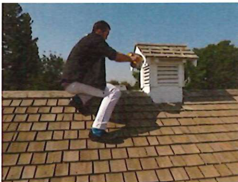
Site testing for lead in paint using a XRF (X-Ray Fluorescence) analyzer
