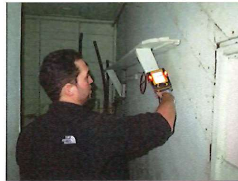
Site testing for lead in paint using a XRF (X-Ray Fluorescence) analyzer
